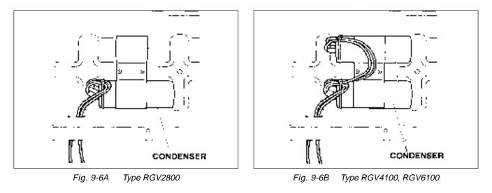
NOTE : Be sure to discharge condensers by shorting condenser leads each other before checking their capacitance, or the accurate reading cannot be obtained.
